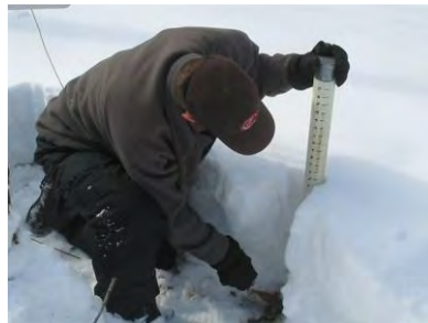
Obtaining snow depth and core sample
