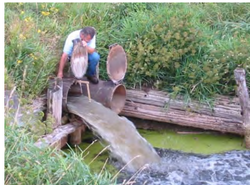
Measuring flow using manual method
