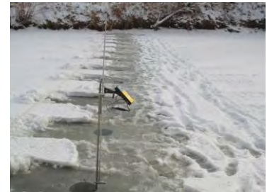
Measuring flow beneath ice
