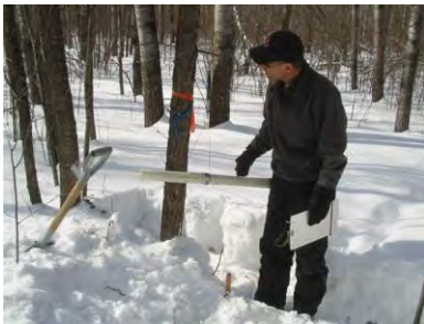
Establish base weight of empty sampling tube
