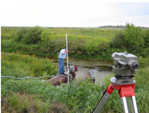
Surveying water lift from river to pump
