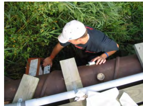
Measuring flow using Doppler method
