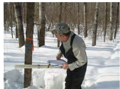
Establishing weight of snow sample to obtain water content
