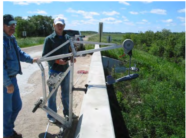
Measuring flow with bridge crane
